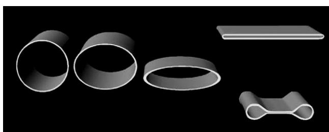
Fig. 37. Modes of collapse of electrospun tubes of polymer into ribbons. Reproduced with permission from Koombhongse et al. [46]. Copyright 2001. John Wiley & Sons, Inc.
